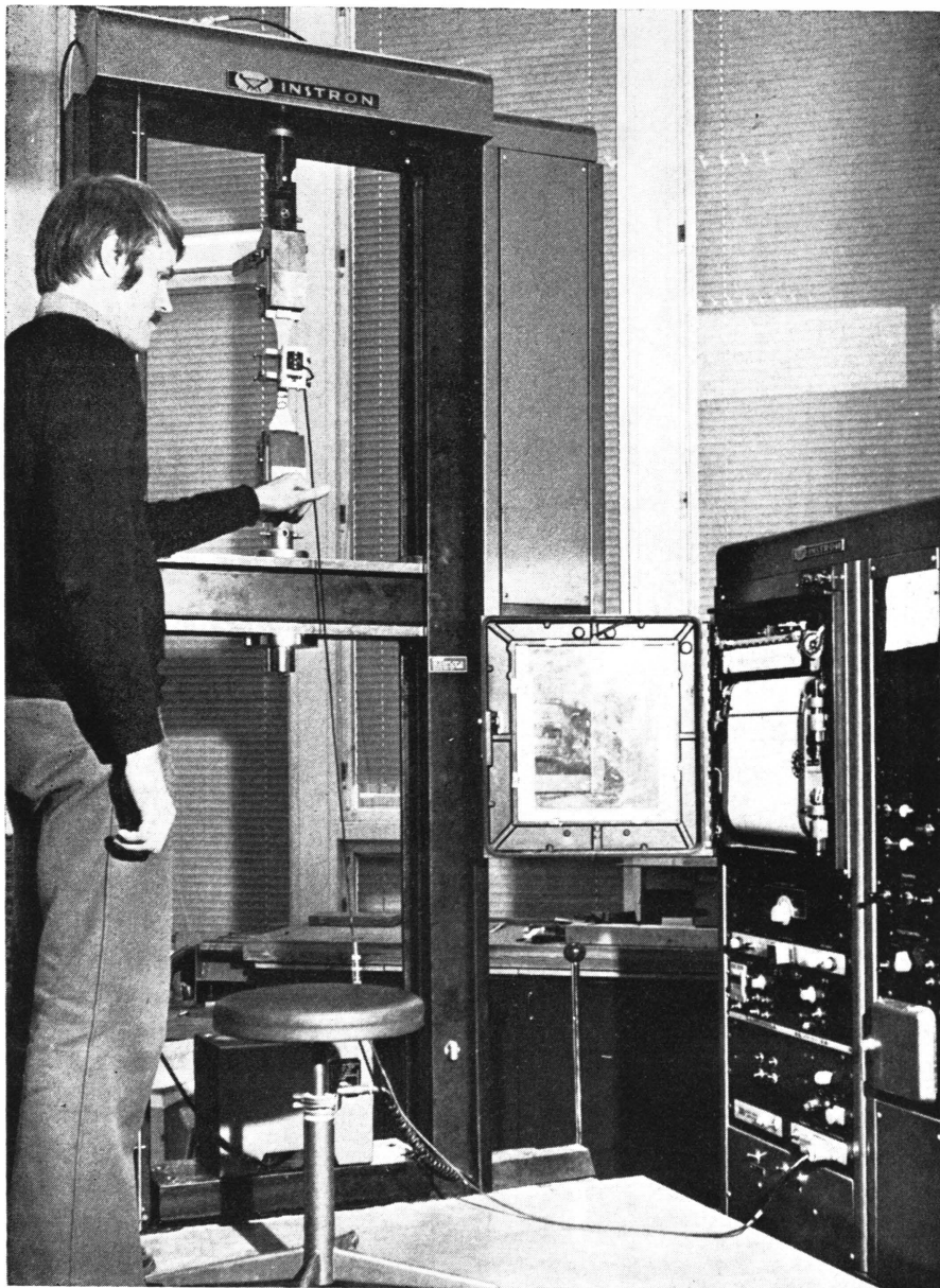
With electronic measuring devices the determination of different strength and elasticity characteristics of wood and wood products is fast and accurate. This illustration shows how the stress-strain diagram of a plywood specimen in tension test is automatically recorded during the progress of the test.
