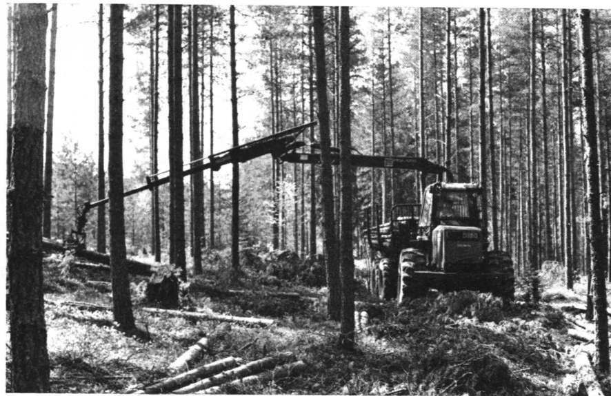
Metsäteho also participates in the development of harvesting machines and equipment. To lighten the work of manual bunching in thinnings long-reach loaders which can be used on medium-sized forwarders have been developed.
