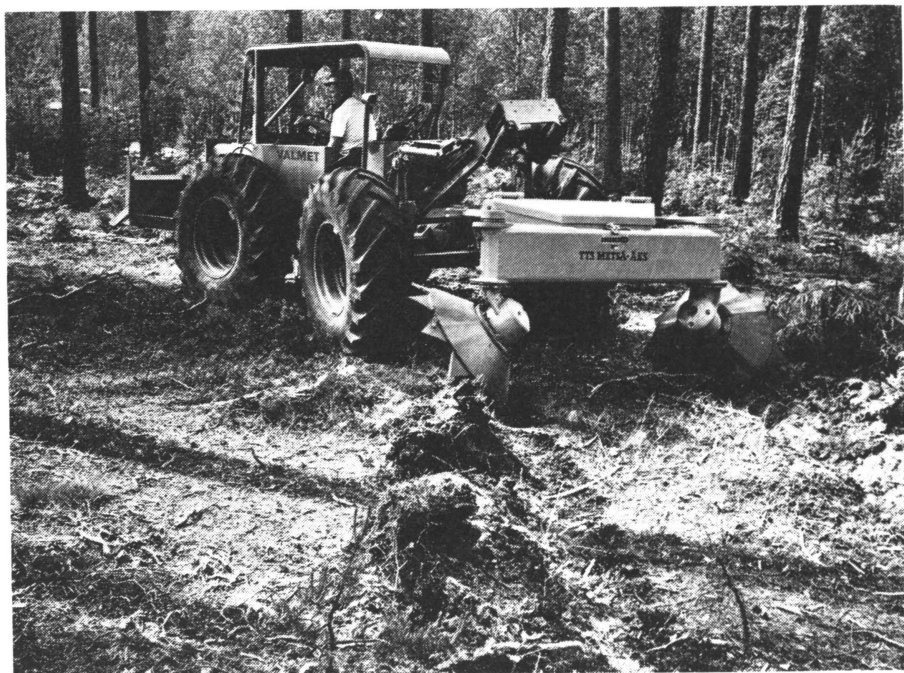
An essential part in the activity of the Work Efficiency Association is to develop working methods and machines. In the picture the TTS-Disc-Trencher for soil preparation.
