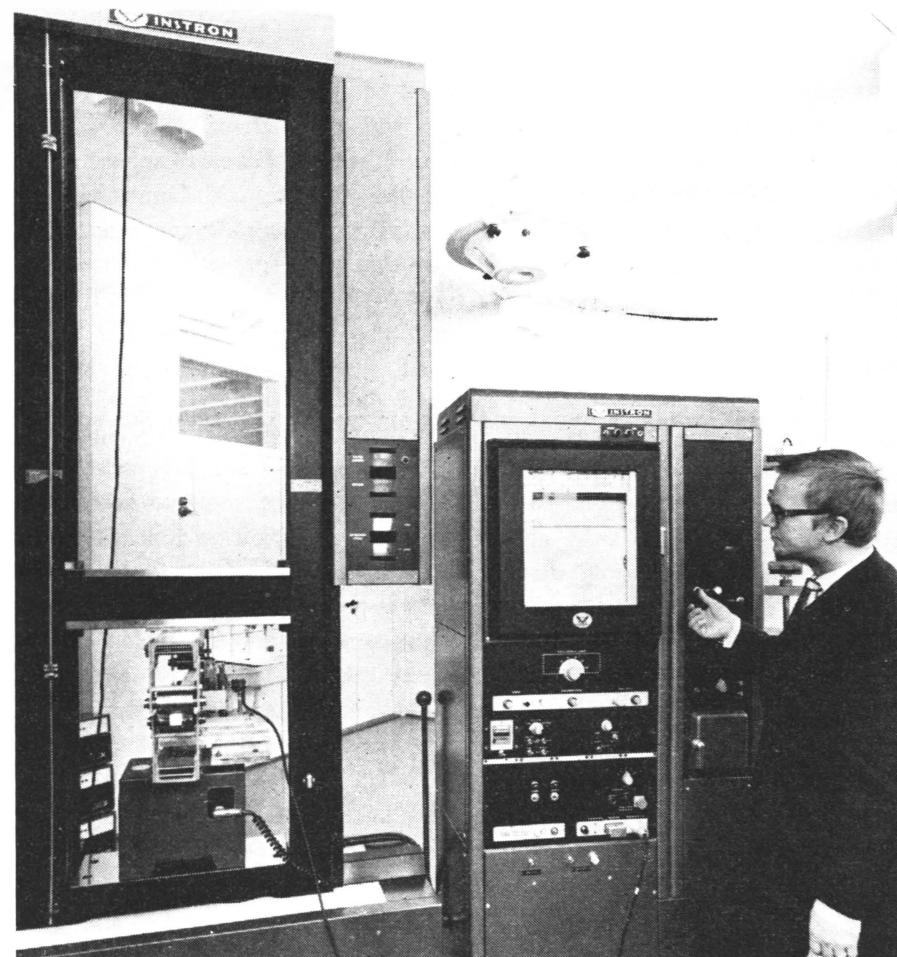
With modern electrical measuring devices, the determination of different strength and elasticity characteristics is fast and accurate. This illustration shows how the stress-strain diagram of the bending test is produced automatically during the progress of the test.
